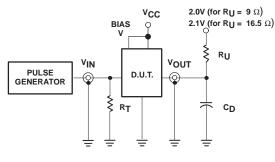
Test Circuit for Outputs on B Port
